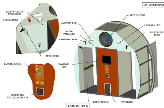
Figure 5 Detail of a cross-connection module
