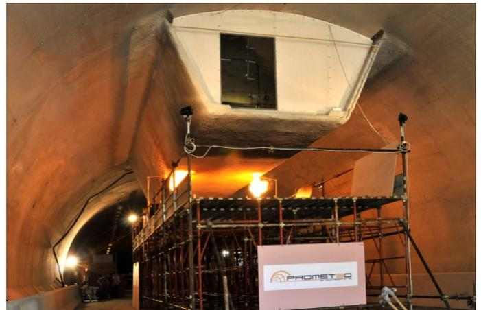
Figura 4 The suspended emergency exit during the fire test
