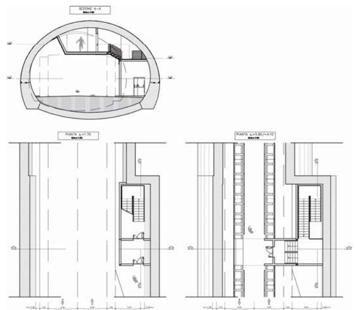
Figure 3 Access inside a section of the tunnel
