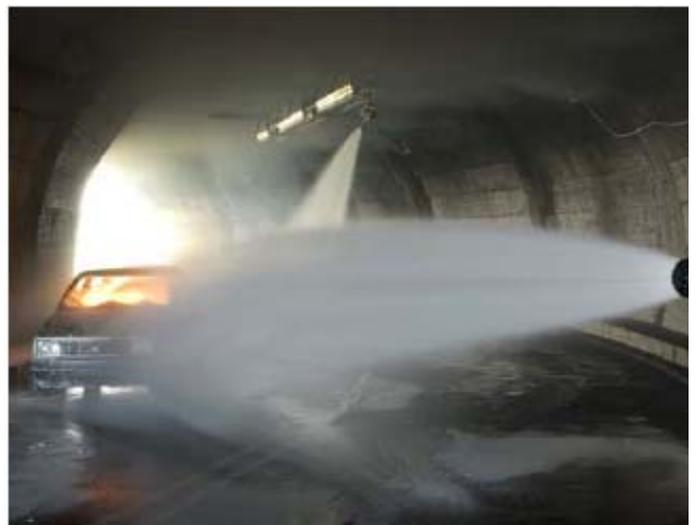
Figure 10 The fire fighting system in action
