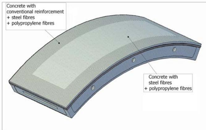
Figure 14 Design solution for segments with optimised conventional + fibre reinforcement
