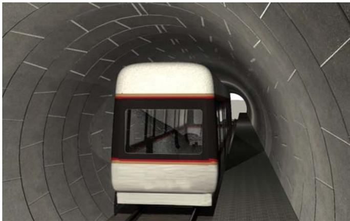
Figure 8 A three dimensional model of the body of a carriage from Line C of the Rome Metro
