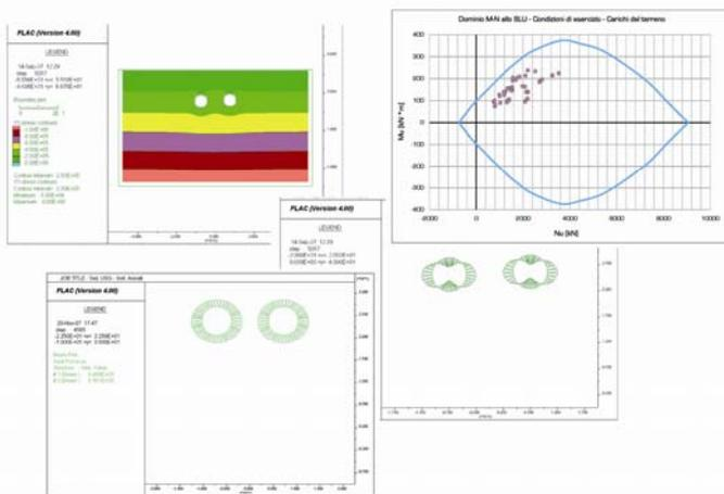
Figure 15 Verification of a section of concrete segment with reinforcement optimised for loads from the ground
