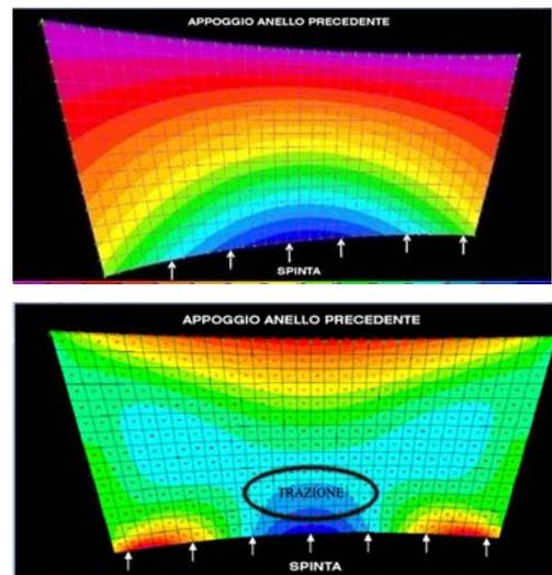
Figure 5 Ideal thrust conditions – Deformation a stress perpendicular to the direction of thrust
