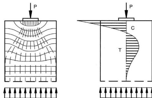
Figure 6 Stress state due to the concentration of a compressive force
