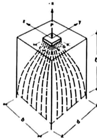
Figure 7 Bursting stresses - 3D stress state
