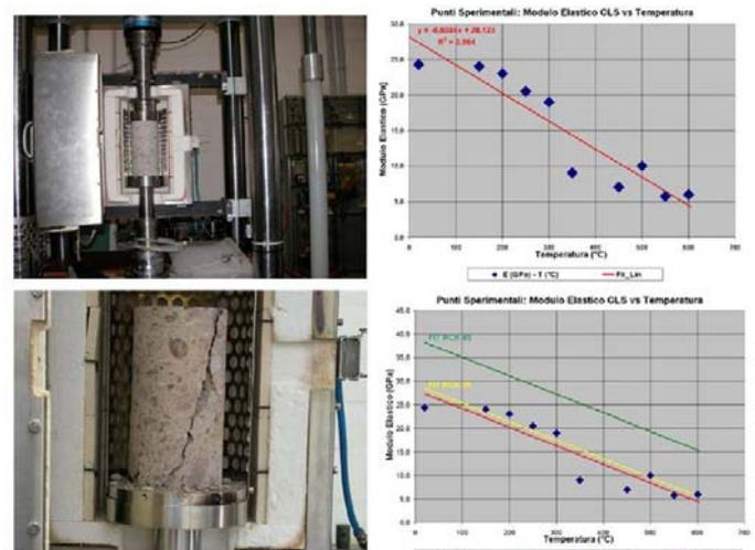
Figure 10 Experimental tests – Changes in the strength characteristics of the materials with temperature
