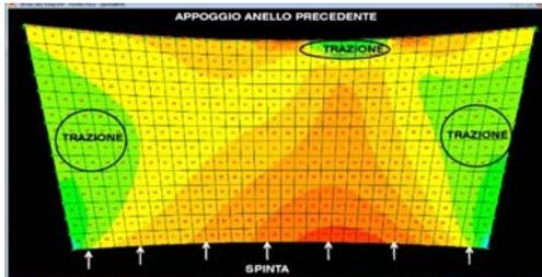
Figure 7 Thrust conditions with assembly defects – Deformation and stress perpendicular to the direction of thrust
